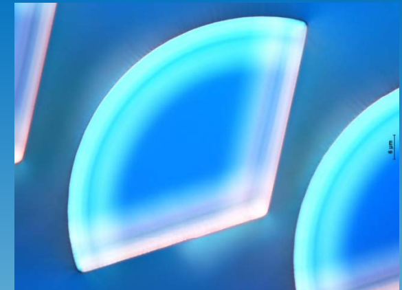
Fig 4: SU-8 triangle shaped compound, angle of 120°
